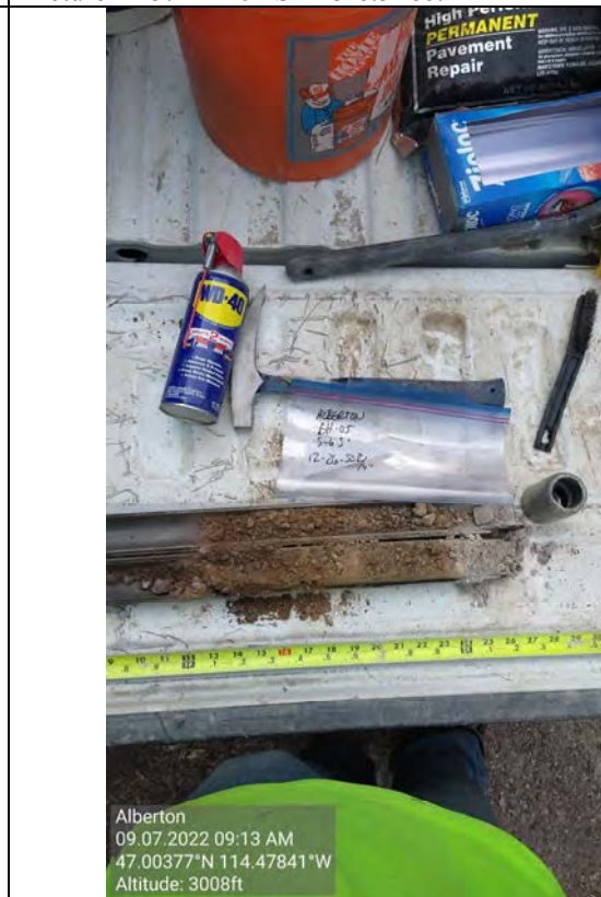
Picture # 17: BH-05 SPT 5-6.5 feet
