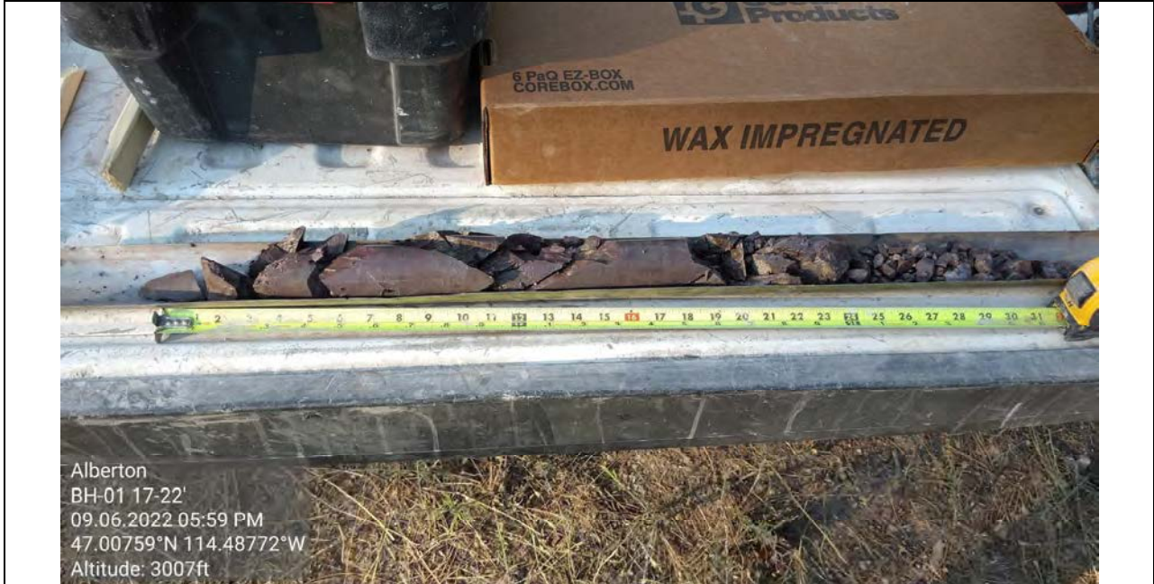
Picture # 7: BH-01 Rock core sampled from 17-22 feet below ground surface
