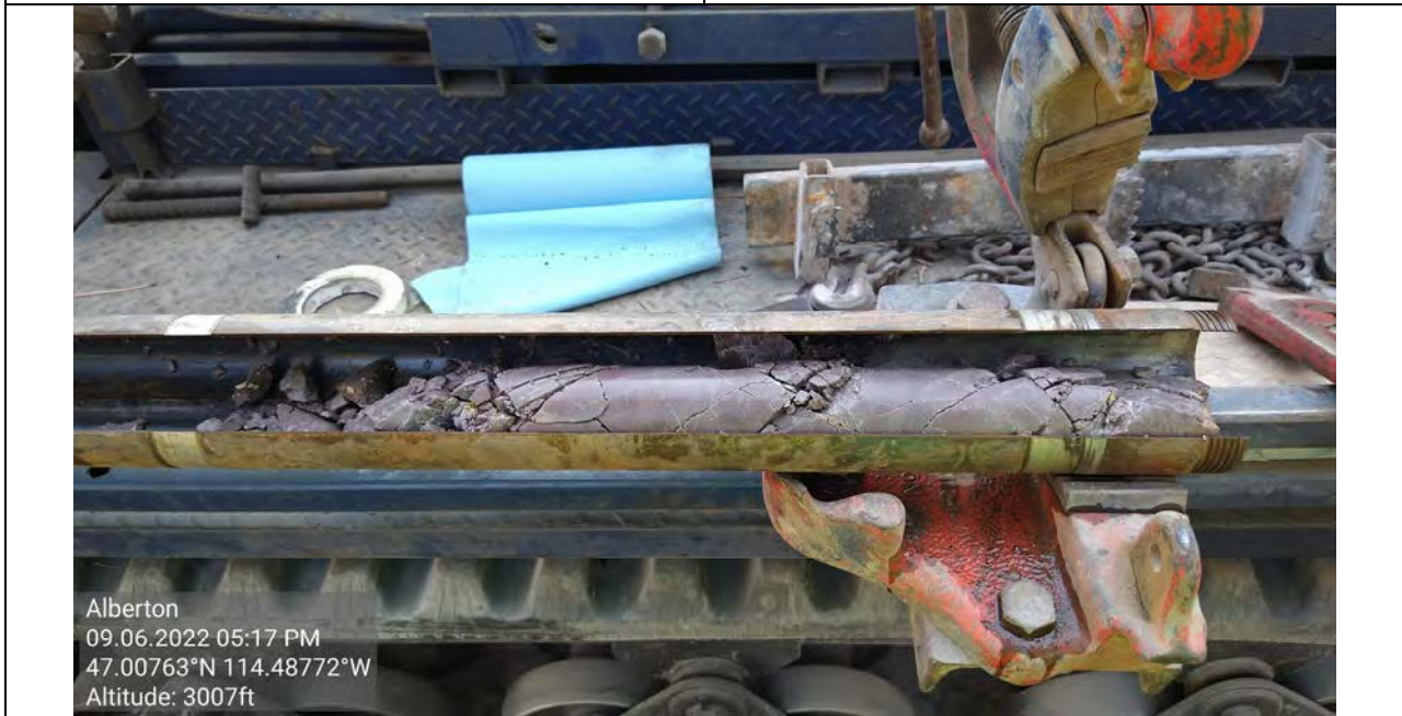
Picture # 6: BH-01 Rock core sampled from 15-17 feet below ground surface
