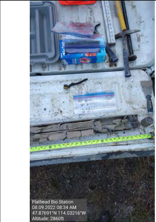
Picture # 14: BH-02 SPT from 10-11.5 feet
