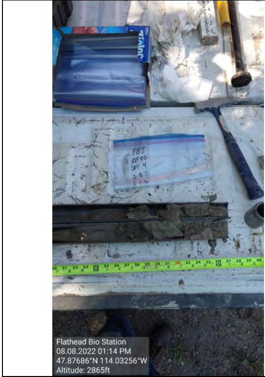
Picture # 7: BH-01 SPT from 15-16.5 feet
