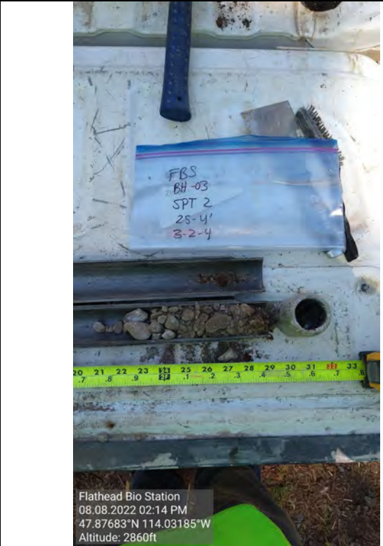
Picture # 22: BH-03 SPT from 2.5-4 feet
