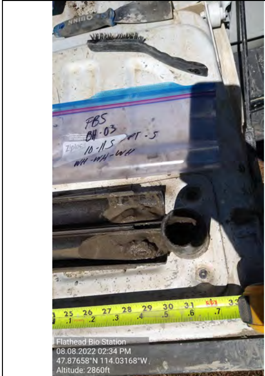
Picture # 25: BH-03 SPT from 10-11.5 feet
