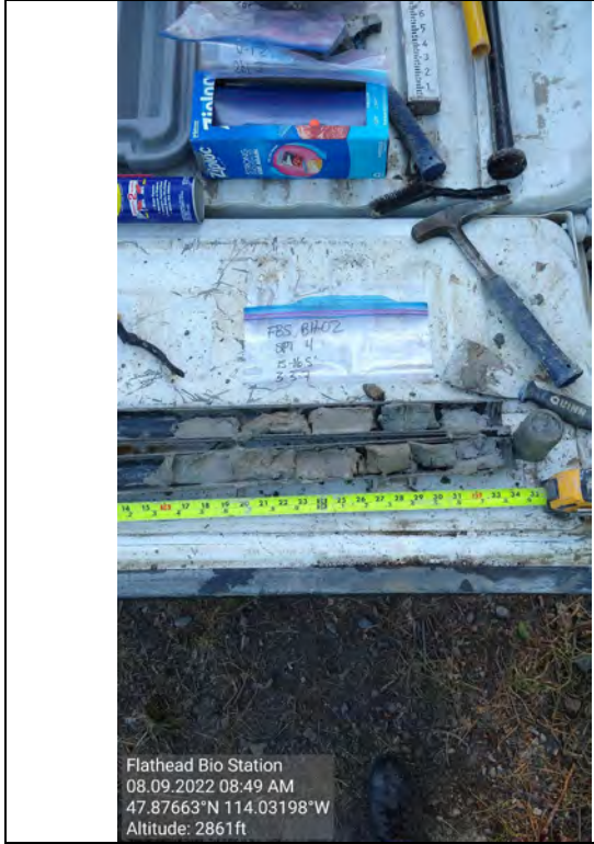
Picture # 15: BH-02 SPT from 15-16.5 feet
