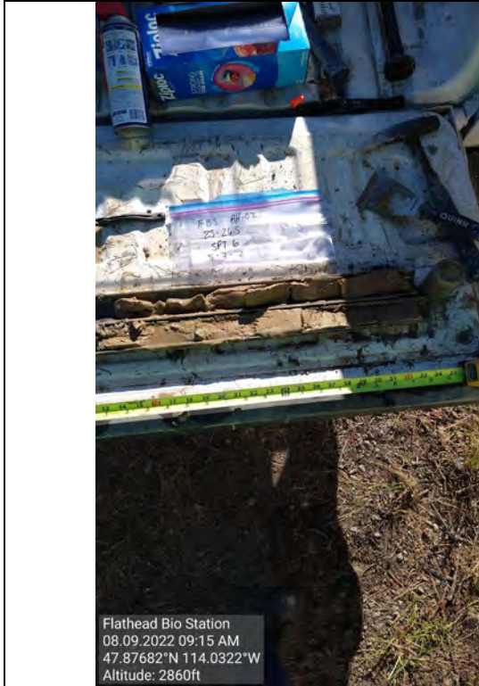
Picture # 17: BH-02 SPT from 25-26.5 feet
