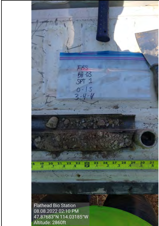
Picture # 21: BH-03 SPT from 0-1.5 feet
