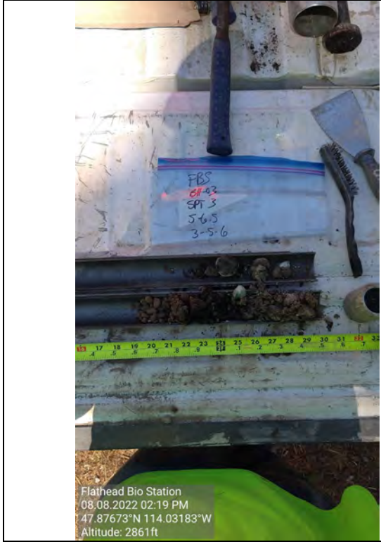
Picture # 23: BH-03 SPT from 5-6.5 feet
