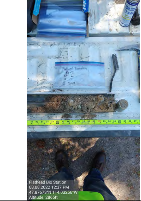
Picture # 4: BH-01 SPT from 0-1.5 feet
