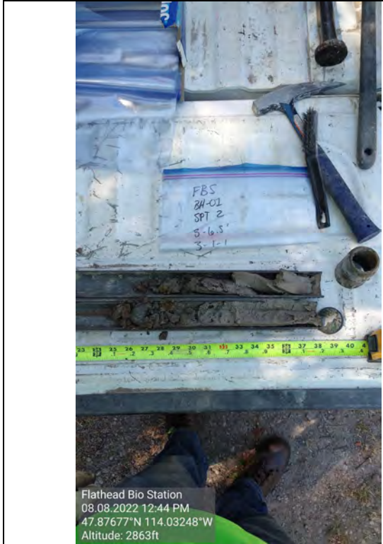
Picture # 5: BH-01 SPT from 5-6.5 feet
