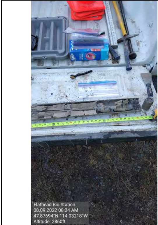
Picture # 13: BH-02 SPT from 10-11.5 feet
