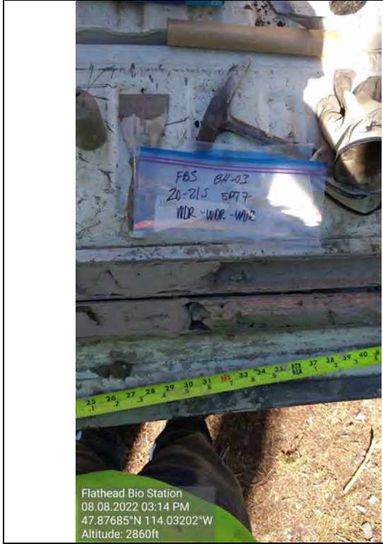
Picture # 27: BH-03 SPT from 20-21.5 feet
