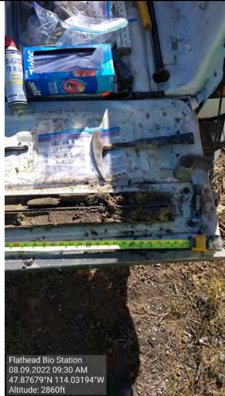
Picture # 18: BH-02 SPT from 30-31.5 feet.
