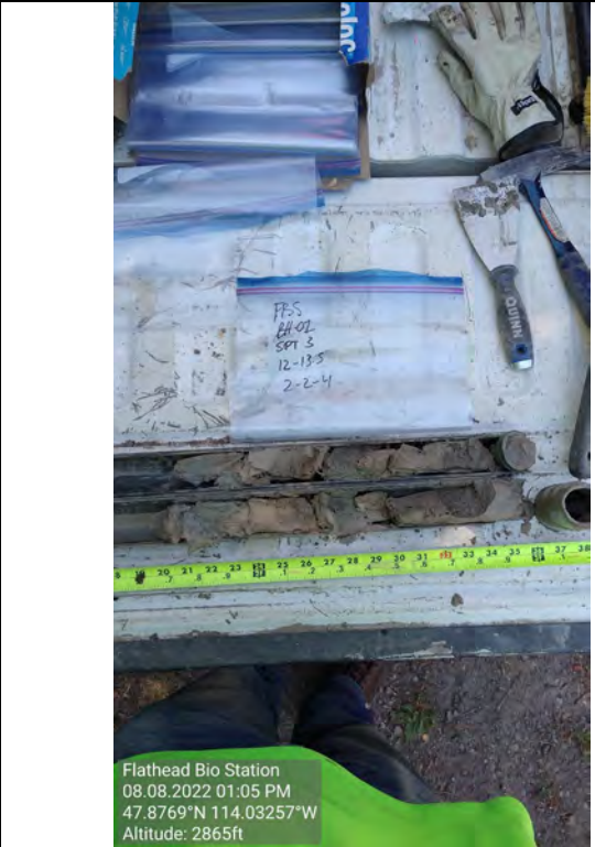
Picture # 6: BH-01 SPT from 12-13.5 feet
