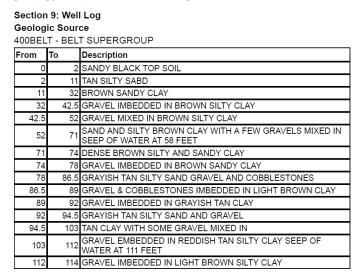
e. geologic conditions affecting the site, such as anticipated interference between proposed and existing wells; The Engineer's subconsultant, Water Environment Technologies, has conducted a well pump test on the existing supply well and monitoring surrounding private wells in order to determine aquifer characteristics. <u>A new well has been sited, but budgetary constraints and indecision regarding a new well vs. spring source have postponed drilling a new well.</u>
