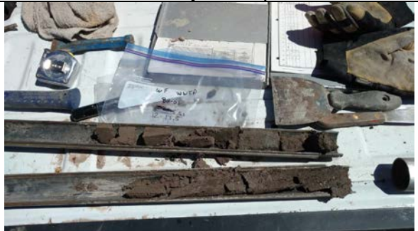
Picture # 4: BH-01, 12' sample interval
