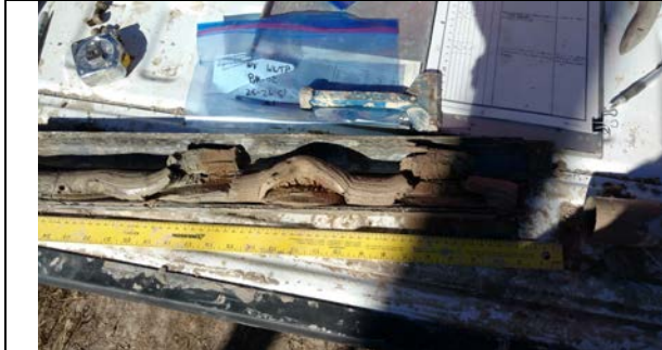
Picture # 19: BH-02, 25' sample interval
