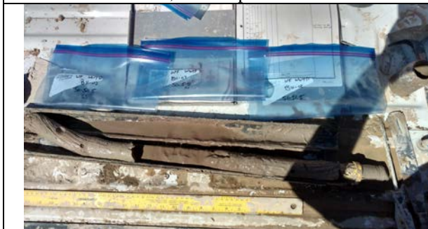
Picture # 23: BH-02, 50' sample interval
